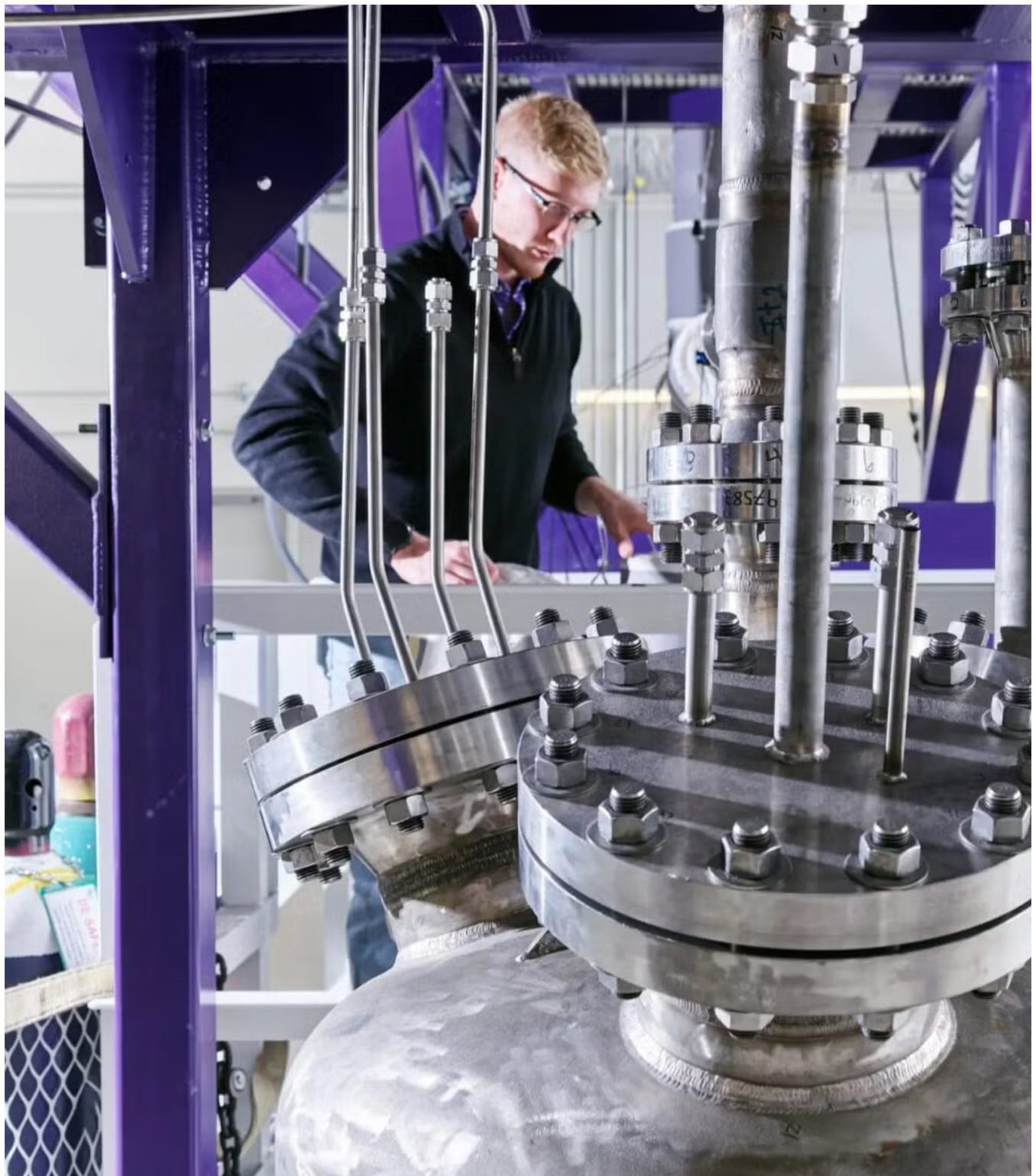
Molten salt test system drain tank. Natura Resources Photos.
